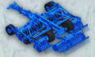
U 652 trailed with a hydraulically foldable frame
