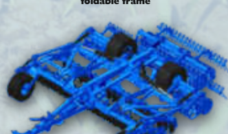
U 652 trailed with a hydraulically foldable frame
