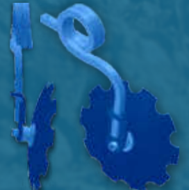
3D spring shock absorber 35x35mm used in U 652 machines
