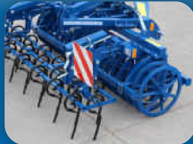
Cambridge roller on the front tractor three-point linkage equipped with a two-row cultivating extension with SU straight spring tines + optional auxiliary spring
