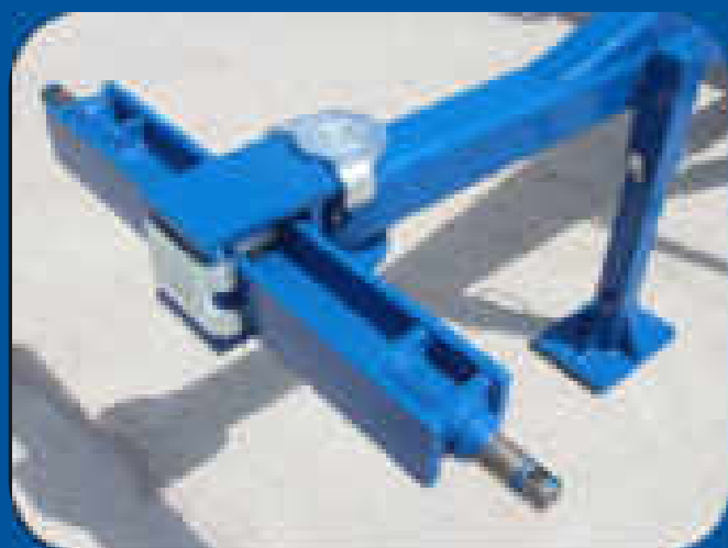
The frame of 4.0m and 4.5m width machine in hydraulically folded version consists of two parts, but the larger frames are divided into three parts.
