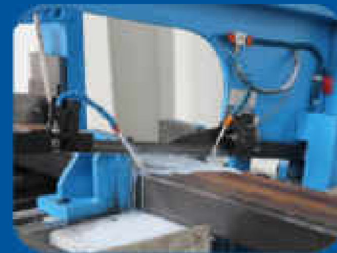
The profiles are cut on precise CNC band saws.
