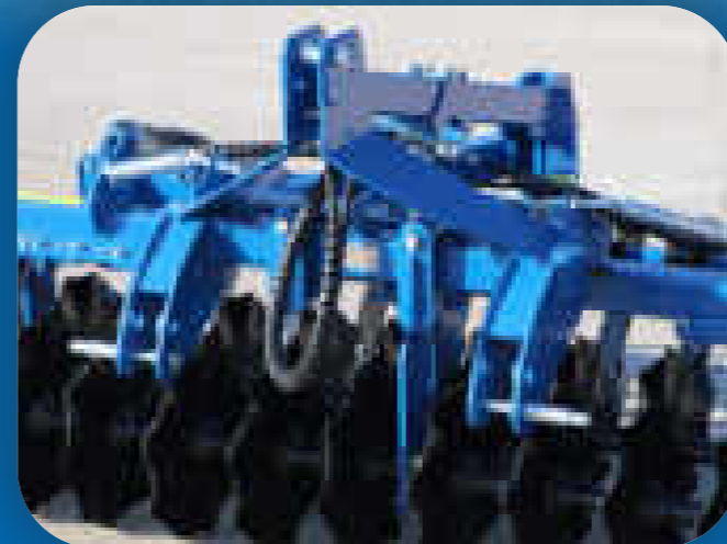
Cambridge roller on the front tractor three-point linkage equipped with a two-row cultivating extension with SU straight spring tines + optional auxiliary spring
