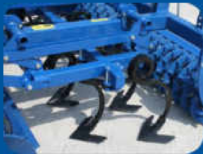
Spring plow beam of 25x25mm section and 260mm wide coupler is a working element designated as SG symbol. This tine is ideal for the work in autumn.
