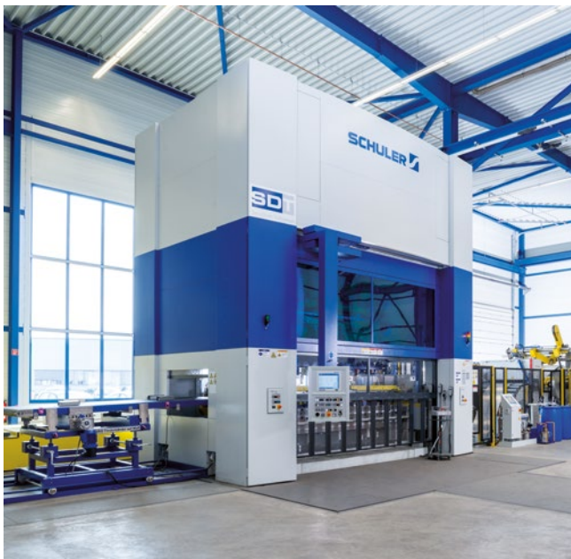
Servo presses in monoblock design in the Process and Technology Centre ProTec, Lennestadt. Press force: 6,300 kN.
