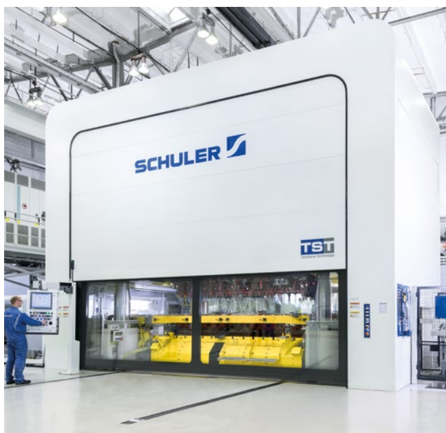
Transfer press with TwinServo Technology at the Schuler Servo TechCenter Erfurt, Germany.
