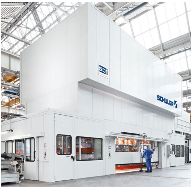
Servo press in tie rod design for a manufacturer of household appliances. Press force: 16,000 kN.
