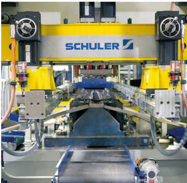
Tri-axis transfer with servo drive »Power Trans«.
