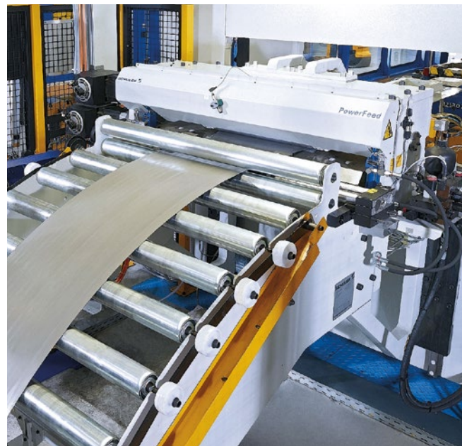
Highly dynamic roll feed »Power Feed«.
