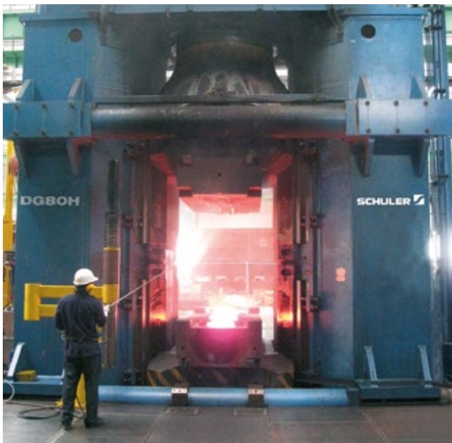
Counterblow hammer with 800 kJ working capacity.
