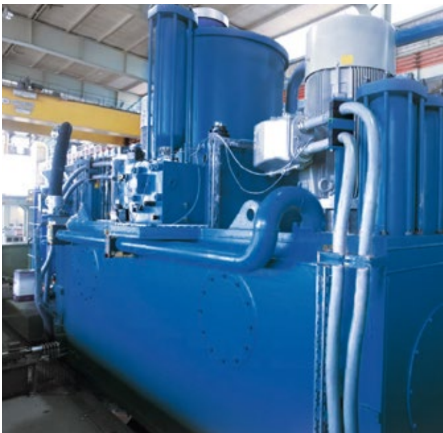
Drive head of a hydraulic counterblow hammer.
