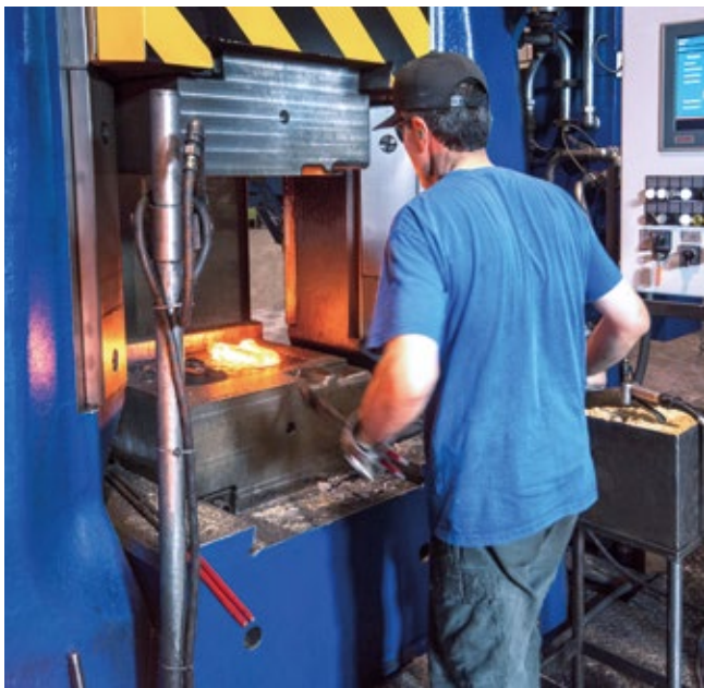
KGH 4 down stroking hammer with proportional valve technology used in forging.
