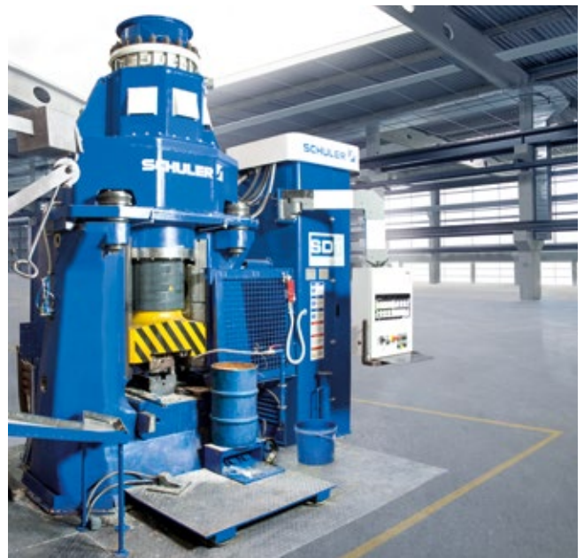
Linear hammer with ServoDirect Technology.
