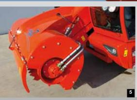
5. Tillaging roller diameter 400 mm, driven by 2 hydraulic motors, power 110 kW, rotation speed 0:670 rpm.
