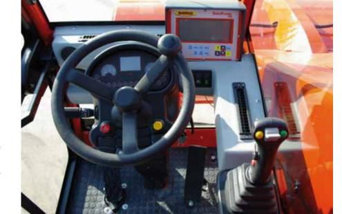
Dependable and advanced weighing and data transfer systems allow programming of different recipes according to the different types of livestock, and constant monitoring of the ration in the display and in the farm management system.
