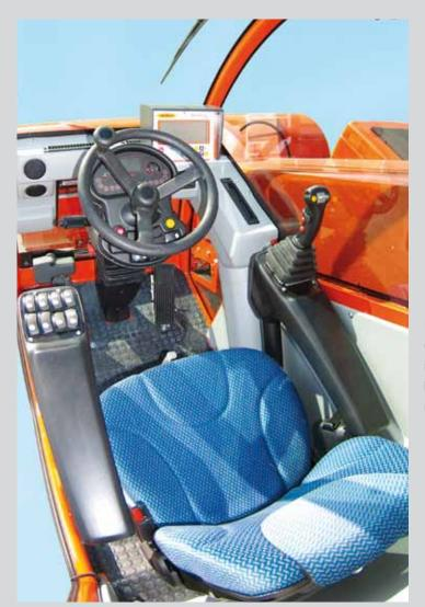
For greater driving comfort, all the main controls (travelling transmission + silage tiller operation) have been incorporated in a practical joystick integrated in the right-hand arm of the seat, while all the manual controls of the machine are operated from the left-hand arm.
