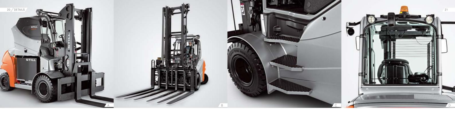
**/ A Lateral battery changing.** Ready for use around the clock – even in multi-shift operation. The battery can be changed laterally quickly and safely at any time without the need for an overhead crane.
