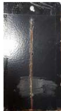
... scatched after 750 h Saltspray-test
