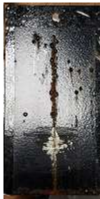
... scatched after 750 h Saltspray-test
