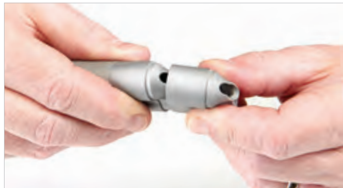
Snap Apart Each Part of the Baffle Stack
