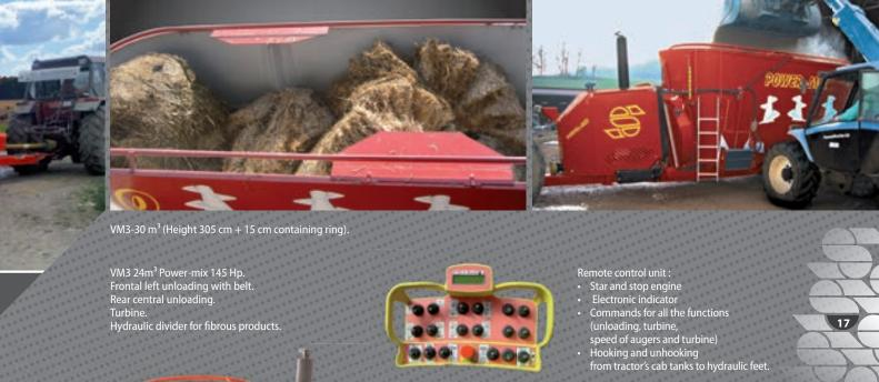
VM3 24m³ Power-mix 145 Hp. Frontal left unloading with belt. Rear central unloading. Turbine. Hydraulic divider for fibrous products.
