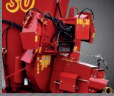
The turbine can be fitted on all versions 2 or 3 augers. Possibility to unloading with the turbine.
