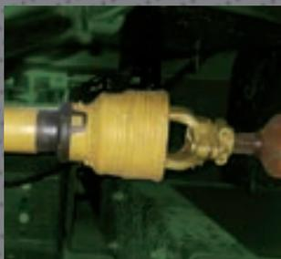
Transmission to the augers by cardan shaft with security bolt.
