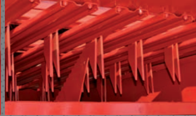
The loading conveyor can be equipped with 5 knives (in the picture only 1).
