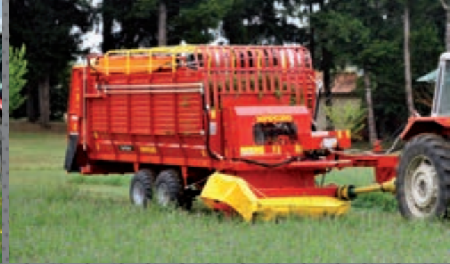
The mowing bar with 2 drums mechanically driven, manufactured by Supertino, allows to work also on uneven grounds.
