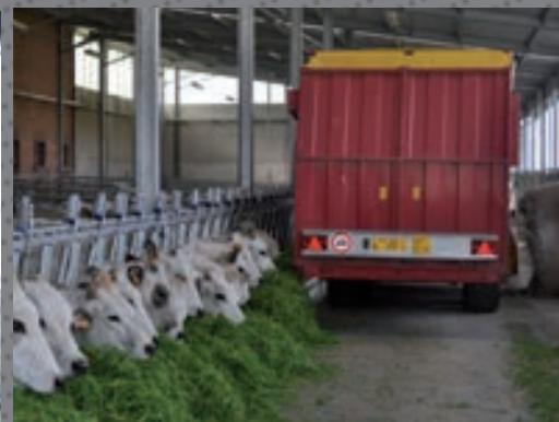
Unloading system with dosing device, 3 rotors and bilateral unloading with belt in PVC.
