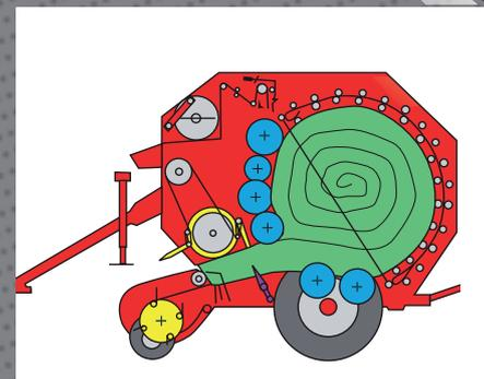
The roller-chain system does not require the disengagement of the PTO at the moment of the opening of the chamber.
