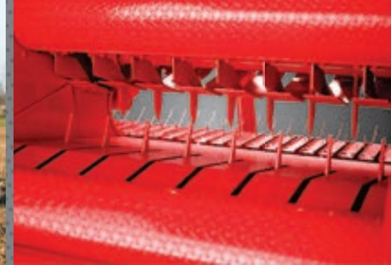
The net binder with direct introduction in the chamber (net is introduced by the rollers) assures tension right from the start of the binding and thanks to the controlled braking system it improves the binding quality of the external borders.
