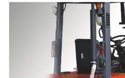
Upward Exhaust Pipe II
