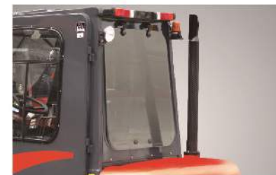
Upward Exhaust Pipe I
