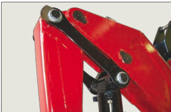
Power link on lifting cylinder
