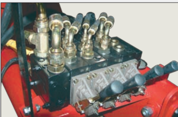
Controls of stabilizers by electro - hydraulic valves Danfoss
