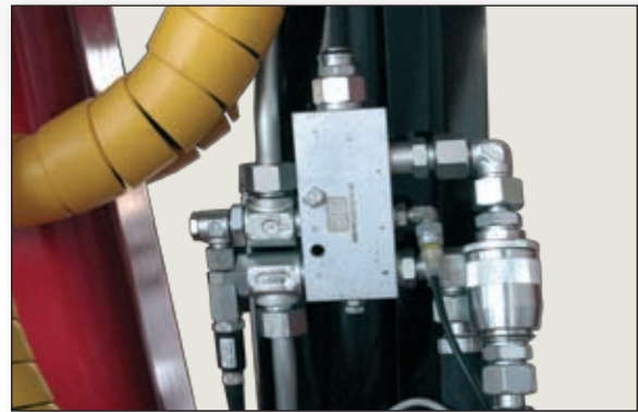
Overcentre valves and rated moment limiter
