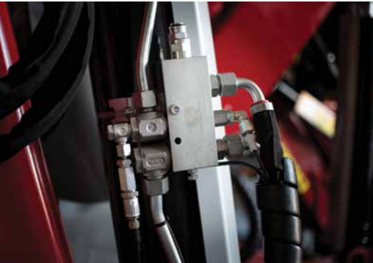
PBC safety box with hour counter enables easier maintenance
