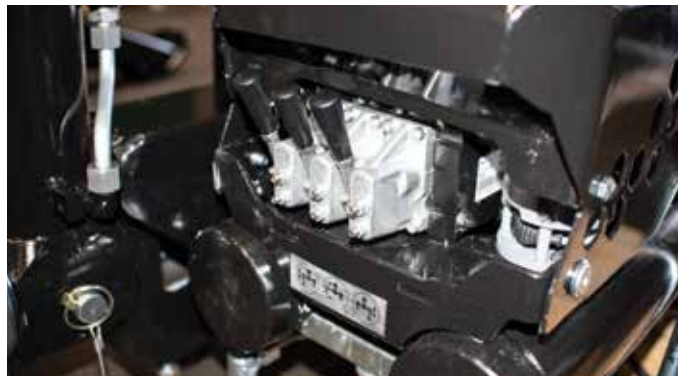
The precise control of outriggers is enabled by Danfoss electro-hydraulic valves. The outriggers can also be operated with the new control console on the seat.
