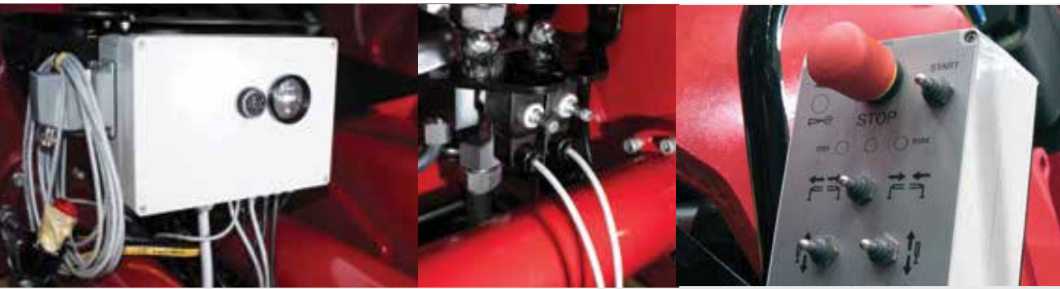
PBC safety box with hour counter enables easier maintenance
