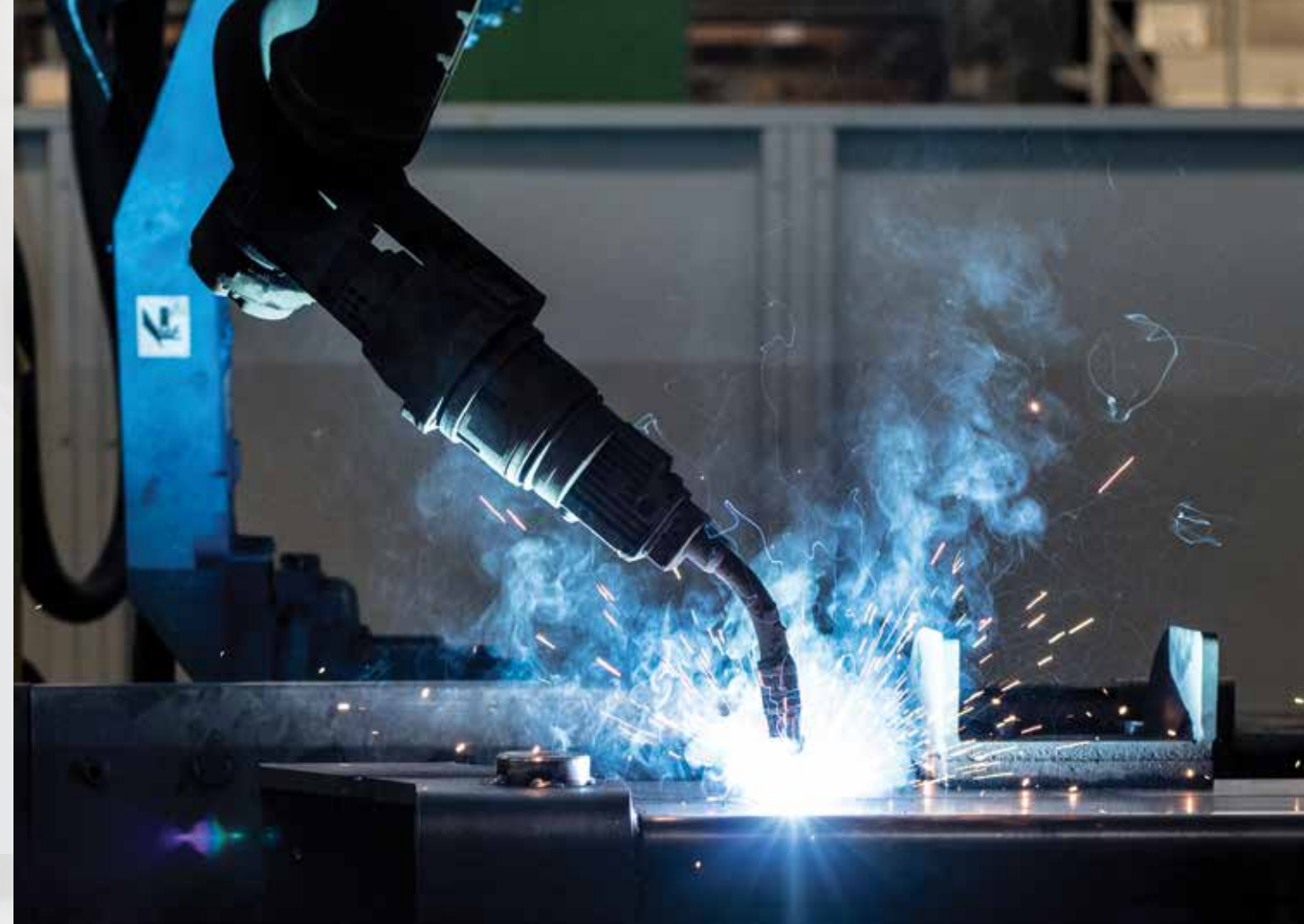
The precise and high-quality welding of hydraulic booms and other parts of the crane using state-of-the-art equipment (Yaskawa).
