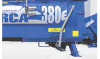
Splitting wedge height is set according to log diameter, using operating handle.
