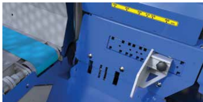
Hydraulic movable limiter is adjustable (7.8"-15.7"). Limiter comes closer for about 1.6" every time the log is forwarding. It returns to its starting position when log forwarding stops. Therefore the cut piece falls safely into the splitting chamber.
