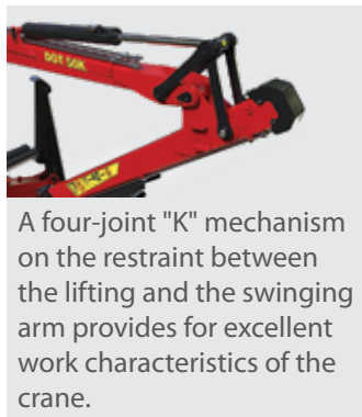
Excellent kinematics of the crankshaft mechanism.
