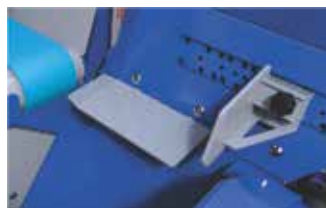
The Swinging Lap remains in the horizontal position during cutting. It helps the last cut piece to fall into the splitting chute in the correct way.
