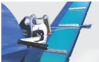
Manual Winch for changing the inclination of the Discharge Conveyor.
