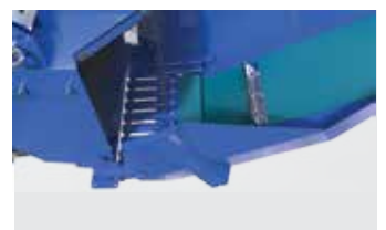
Lattice for Sawdust is located between the splitting wedge and the Discharge Conveyor.
