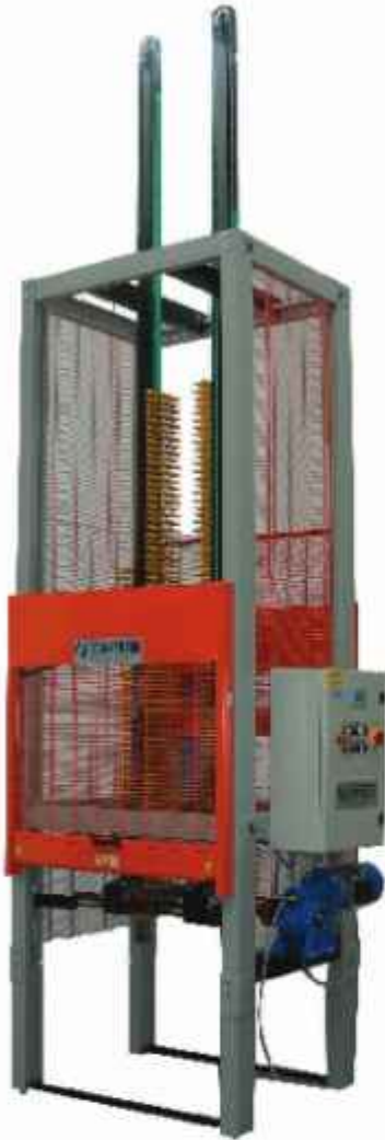
14) CMP – Compensatore verticale ad alette autoregolanti. CMP – Compensatore verticale ad alette. 14) CMP – Vertical compensator with self-adjustable tongues. CMP – Vertical slat compensator.
