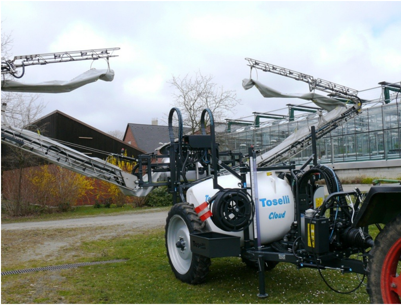
Fig.2: Unfolding of the boom.
