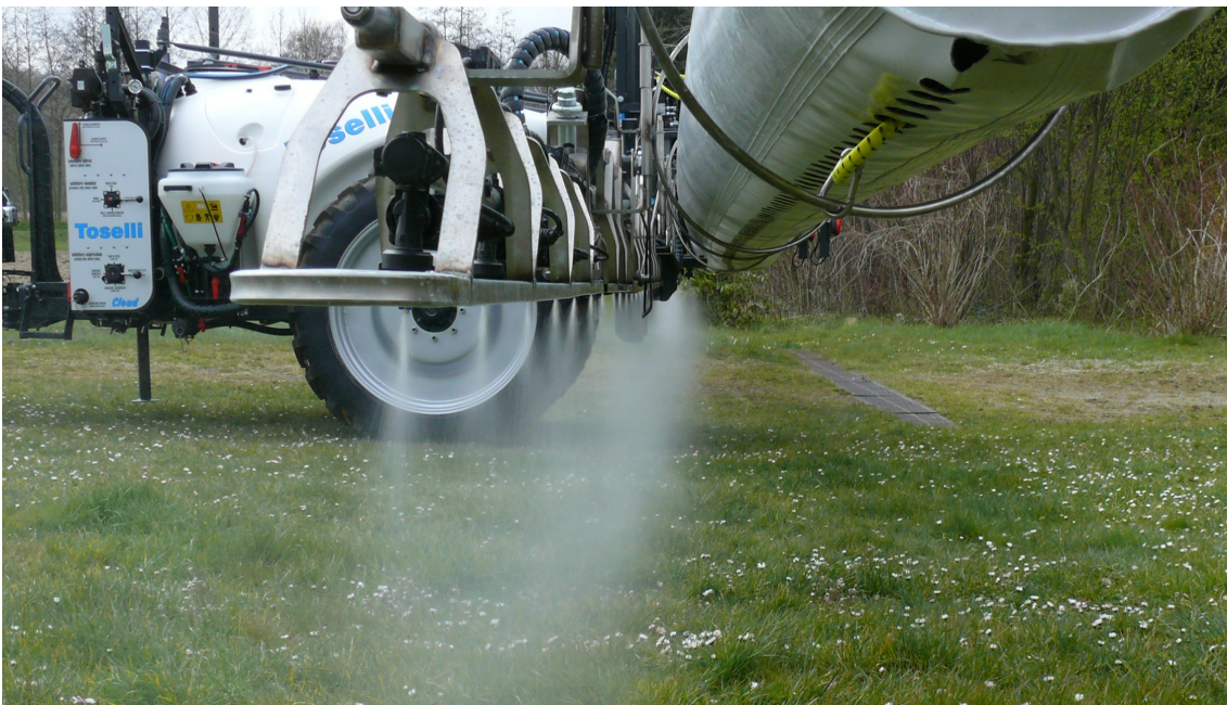
Fig.3: Air assistance tube with outlet openings at the bottom shall increase penetration and reduce drift.
