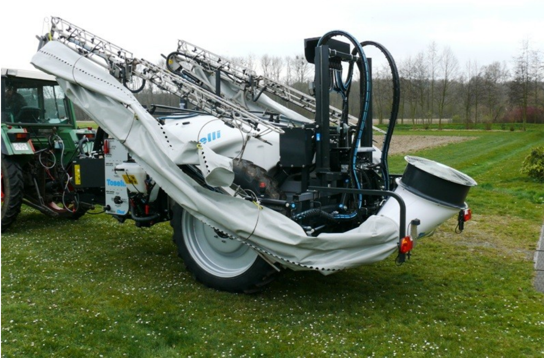
Fig.4: Folded boom with air tube and axial fan (in the rear) for air assistance.
