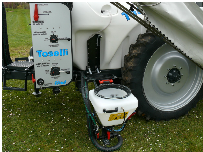
Fig.5: Left sprayer side with induction bowl and control center.
