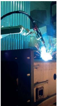
Robotic welding at the hydraulic breaker section provides accurate positioning of parts and no leash, which guarantees 0% defect for 10 thousand units at the output.
