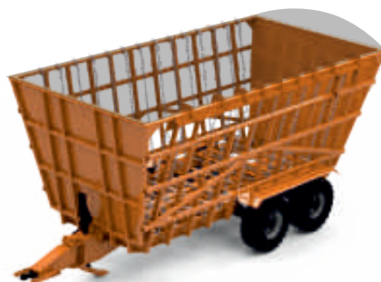
Water filled volumem= 48 m 3 700mm bulged volume = 60 m 3
