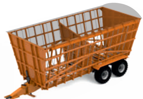
Water filled volumem= 58 m 3 700mm bulged volume = 74 m 3
