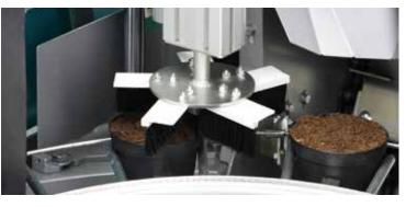
productivity is combined with convenient handling and controls for easy changeover to different pot diameters. The electronic frequency controls for the turntable and elevator ensure precise output control and are easy to operate via the control panel within the working area. Additional frequency converters for soil conveyor, drill motor and conveyor belt are available with surcharge.
