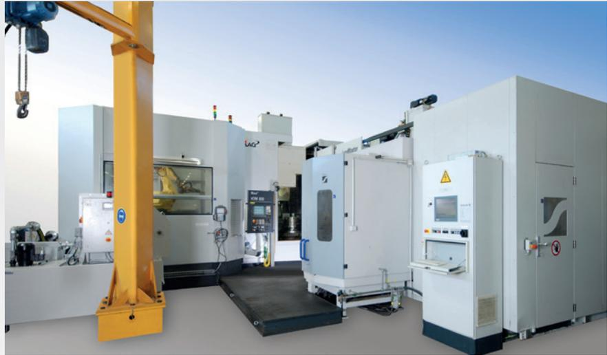
Flexible processing cells with robot assembly and 370 tools
