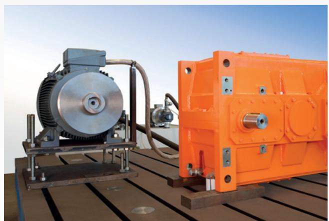
125 kW test bench with closed-circuit oil cooling
