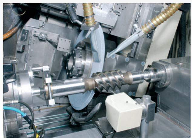
Worm gear grinding
