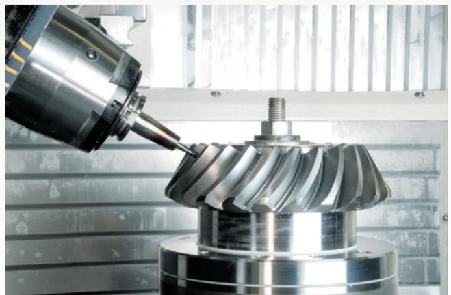
*Five-axis CNC milling - max. Ø: 2800 mm*
