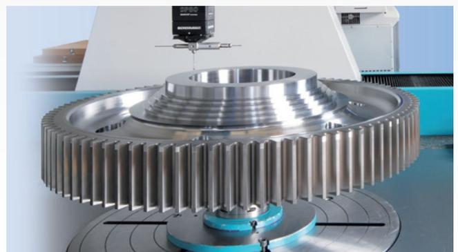
3D measurement of gear wheels
