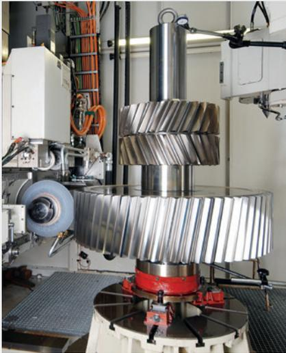
Spur gear grinding up to d=2000mm
