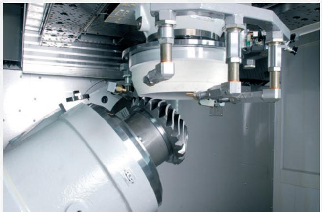
*Bevel gear grinding - max. Ø: 900 mm*
