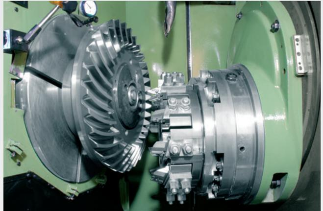
*HPG process / hard machining - max. Ø: 1400 mm*
