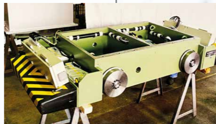
1991 Coil transport car (coil storage to reel)
