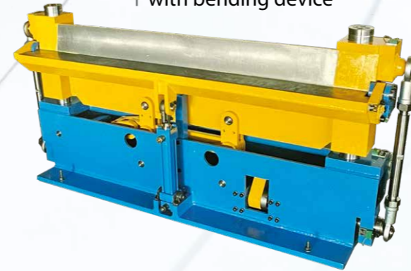
1995 ITT Richter pressing machine for lining housings with PFA, FEP, etc.
