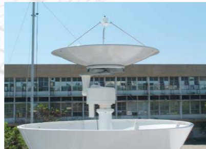
1991 Antenna rotor AR/AE 1021 installed in a radome (Dartcom)
